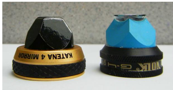
Katena vs Volk 4-mirror gonioscopy lenses (this Volk happens to have a flange, but the no-flange version is similar; the ring to hold the lens is a bit skinnier and the lens is bit shorter than the Katena).
